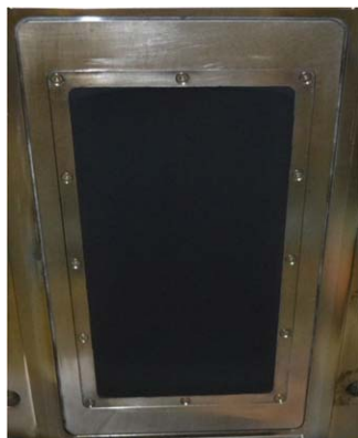
Figure 2. Heat exchanger with plate-catalyst incorporated into upper metal block.
