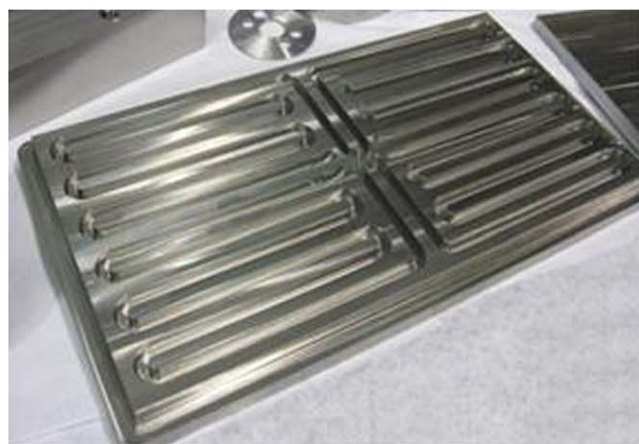
Figure 3. Grooved channels in (a) heat exchanger and (b) lower metal block.
